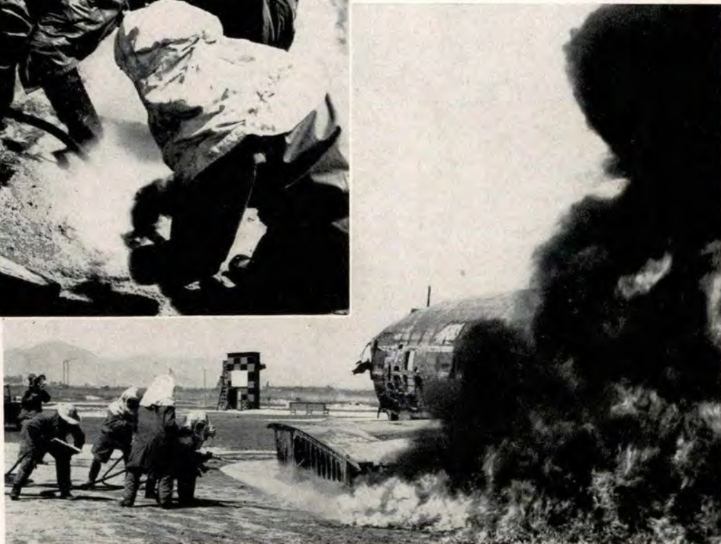
The crash fire fighters' first concern is rescuing the plane's crew-members before an explosion occurs. A spray of water is played on the engines and fuel tanks to keep them cool until the rescue is completed. Then the fire is extinguished.
