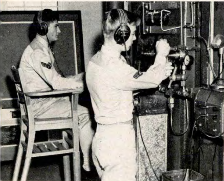
Trained operators at the controls of the Low Pressure Chamber which provides realistic sensations of flights at higher altitudes.
