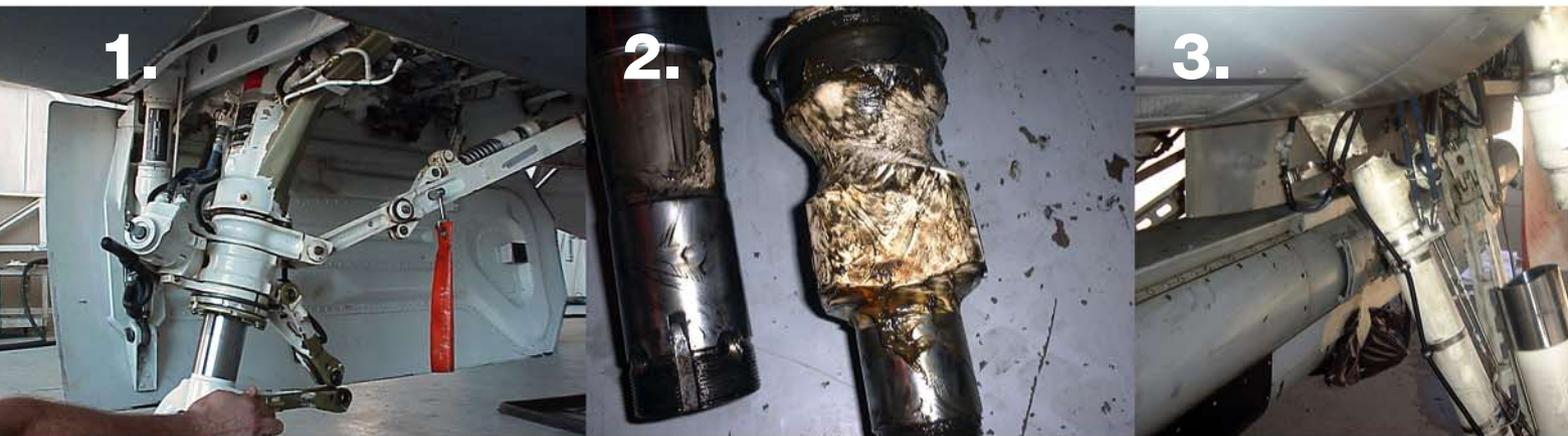
What causes HE in high-strength steel landing gear parts? How about, every @&# thing! Here's a short list: Water (tap and di-ionized), most cleaners on earth (except a tiny handful), rust strippers, every electroplating solution, hoof and mouth disease disinfectants, soft drinks, etc., etc. When steel landing gear parts are exposed to any fluid except authorized cleaning fluids (such as P-D-680), our engineers are programmed to suspect HE and react accordingly.
