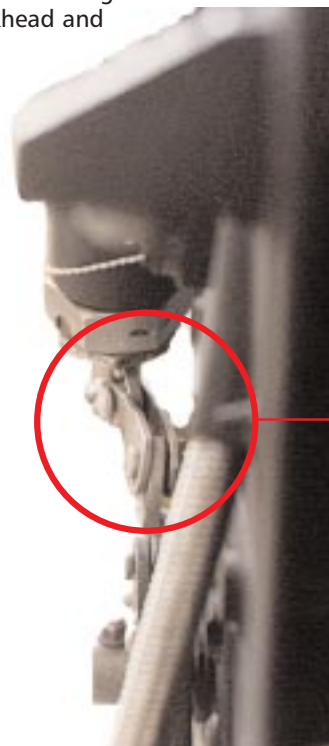
(Left) The ejection-seat guillotine linkage was bent when someone forced the seat up while the lap belt was wedged between the seat and the bulkhead.
