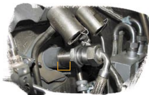
A Improperly Installed Igniter-Left Side
