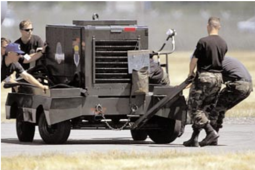
Maintainers on the C-130 ramp muscle a power cart into position after blocking in their aircraft.
