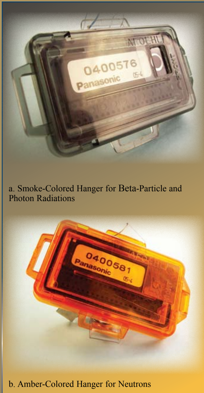
Figure 2: Air Force Dosimeters for Nuclear Weapons Workers and Other Personnel Exposed to Radiation Fields with Photons and Neutrons
