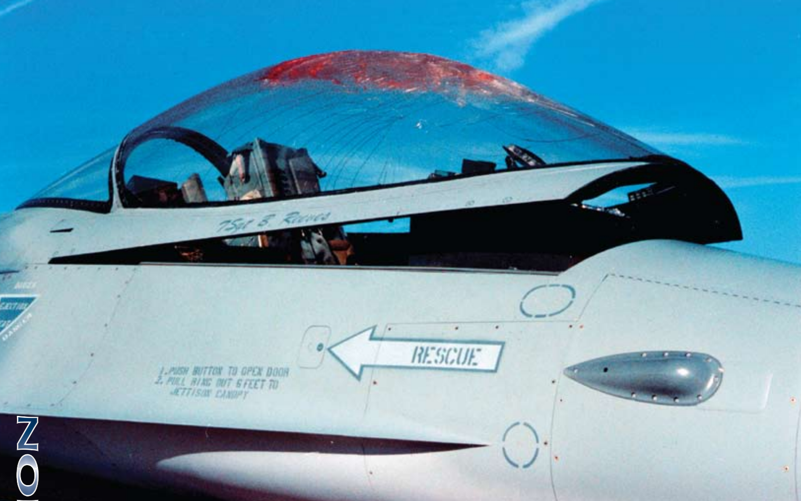
>>> Above: This older F-16 canopy remained intact but still bowed inward from a bird strike. New F-16 canopies withstand 500-plus-knot impacts with 4-pound birds. Opposite: International Flight Safety Officer students inspect a T-38 wing for pre-impact damage.
