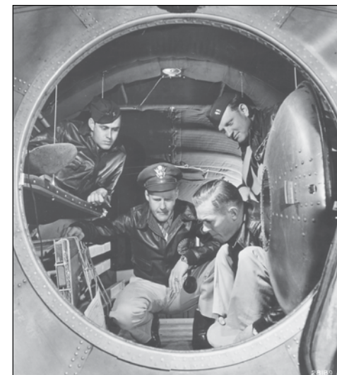
Interior photo of the B-29 Superfortress bomber. Shown is the rear pressurized cabin, equipped with four bunks to give crew members a chance for rest on a long mission. This was an important factor in combating flight fatigue. The B-29 was first reported in action on June 5, 1944, in an attack on railway yards at Bangkok, Siam, and on June 15 the first raid was made in Japan from bases in China. (U.S. Air Force photo)
