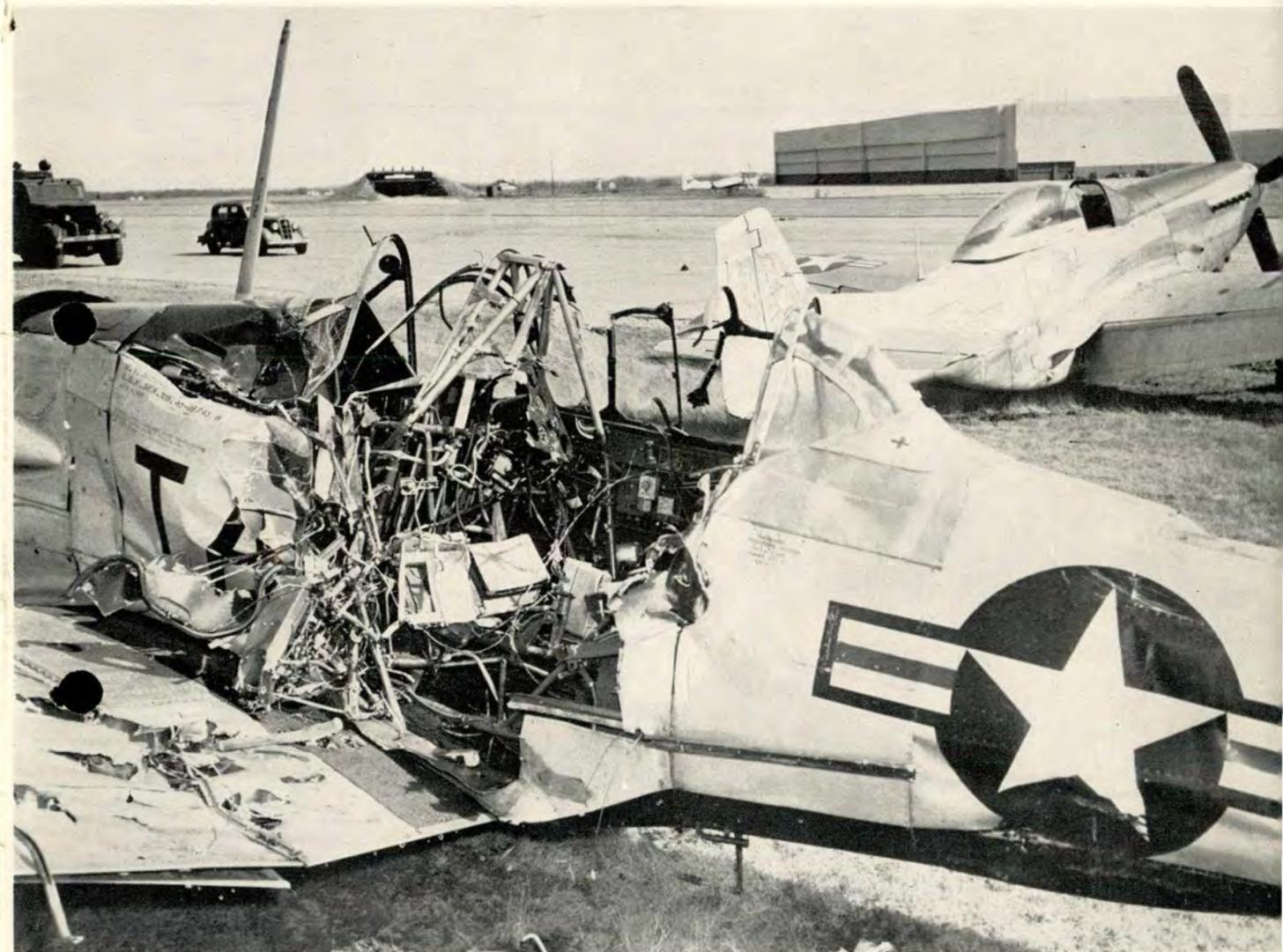
THE PILOT of this P-51 had made several unsuccessful attempts to contact the tower and then made an approach to land still watching the tower for a green light. He failed to see the AT-6 below and in front of him which was also on the approach and had been cleared by the tower to land.
