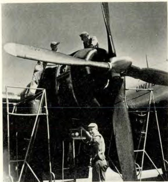
Installing fuel injection pump.
