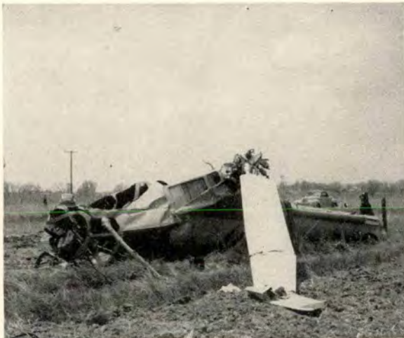
After the blue main rotor blade flew off in flight, one of the remaining blades swung downward smashing the cabin.
