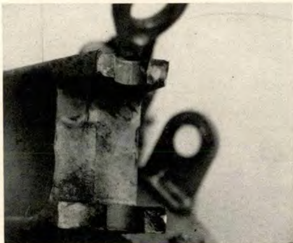
Above: Bearing samples. Below: Old crack evident in upper fitting.
