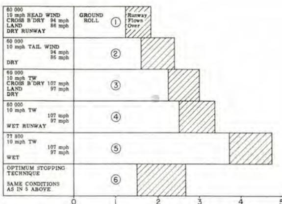
Landing distances under various conditions—Distances (1) through (5) of the above graph indicate the effect of various factors other than pilot technique, upon airplane landing roll. Note that under the assumed conditions, the ground roll distance is almost tripled by the combination of an increase in weight and landing speed, a wind shift, and a wet runway. Although the figures have been determined for a Constellation, they may be considered as representative of any airplane.
