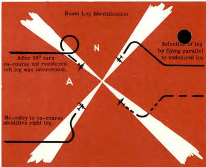
less, a close-in procedure, which will be described later, should be used. If the time is more than seven seconds, a 90° turn to the left is started immediately after receiving the first off-course signal. If within a minute the on-course is not re-entered, and the background signal fades, the beam to the left of the inbound bi-sector heading has been intercepted.
