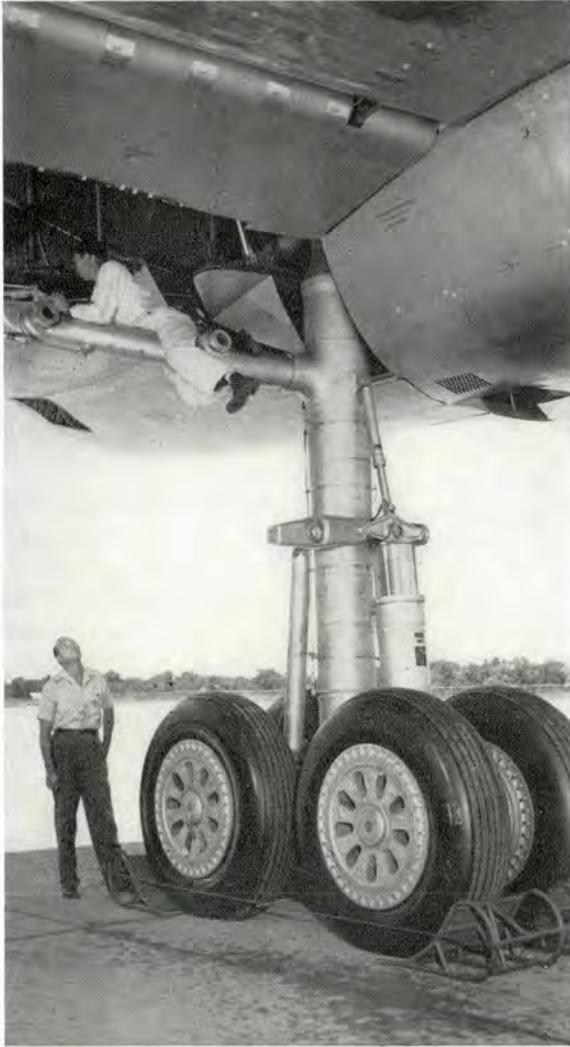
Four wheel main gear distributes B-36 weight. Permits Operation on any runway suitable for B-29's
