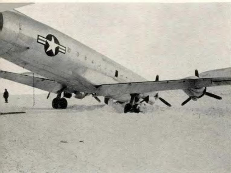
A landing accident near the completion of Project Re-supply happened at Resolute Bay when a C-54 pilot did not correct for cross wind.
