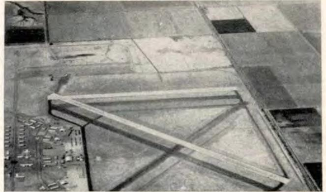
In this un-retouched photo, runways of a desert airfield 43 feet below sea level appear elevated. While this is an optical illusion, high temperatures do have the same effect as elevating runways.
