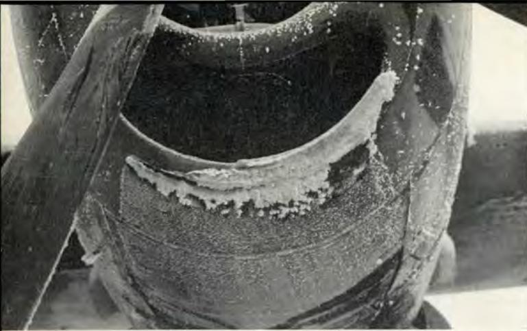
Surface icing is not limited to wings; the nose and underside of your plane can ice up just as easily and you may never know it.
