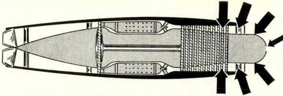
Above, arrows indicate points at which turbojet engines are most susceptible to icing. Designers are at present developing methods of preventing ice formation in these areas and the problem should soon be eliminated.
