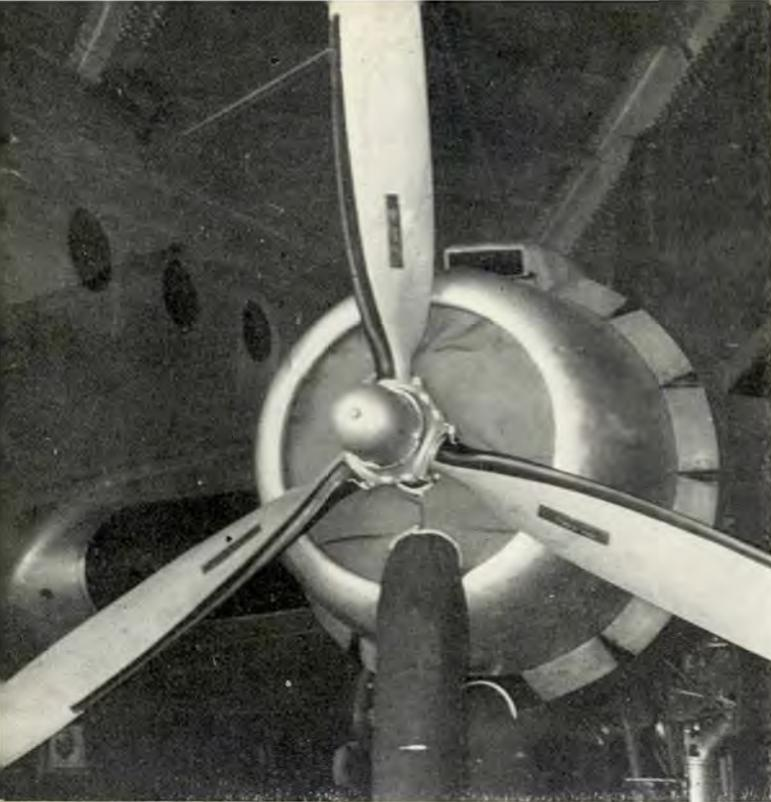
Heating engines before starting is a must in Arctic operations. Above, cowling excluders are used in heating a C-54 engine.
