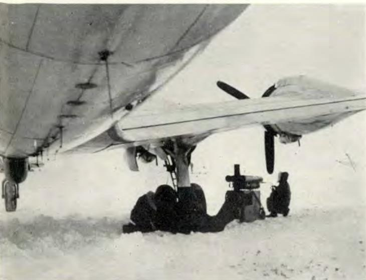
Heating engines and cockpits are not the only uses for heaters. Frozen brakes must be thawed out before the plane can be moved.
