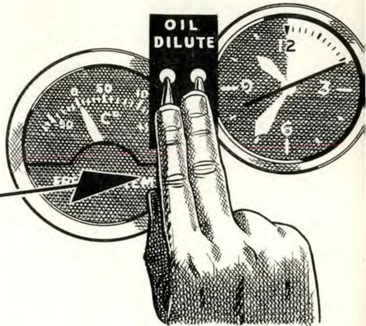
Why dilute engines? The answer is simple. It's to insure that fluid oil will be available for the next engine start. In below freezing weather, undiluted oil may congeal with the result that fluid oil will not be available to provide lubrication when the engine is next started.
