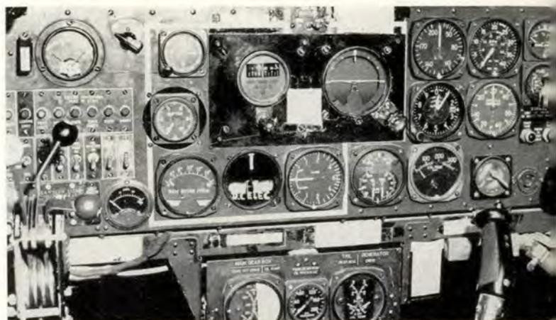
Above, the USAF arrangement has pairs and groups of related instruments along the horizontal axis of the panel. Below is the arrangement of helicopter instruments as currently used by the Los Angeles Airways.
