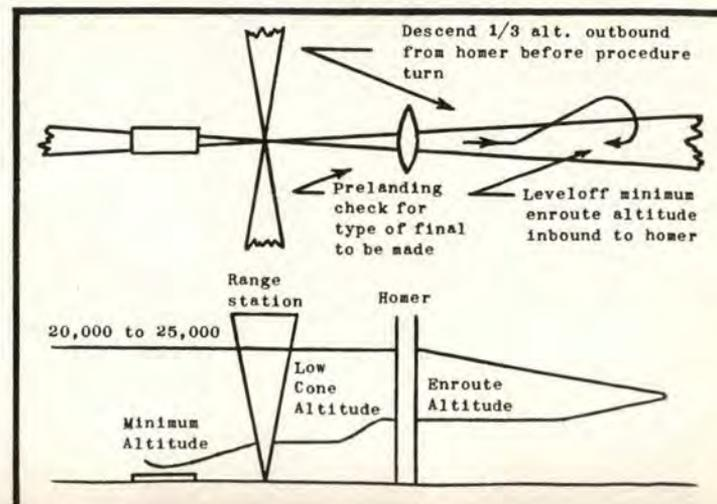
the indicated airspeed to 130 mph (140-145 mph in formation). Add five miles per hour to the above airspeeds for each 100 gallons of fuel remaining in excess of 200 gallons. Descend to the altitude which will intercept the glide path at the proper point. Then adjust the power to maintain altitude and airspeed. The amount of fuel used in this type penetration and low approach for the T-33 is 65 to 70 gallons.
