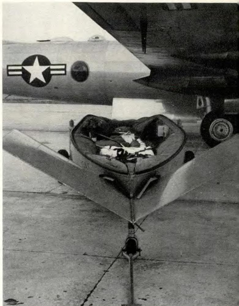
For overwater search, SB-17's are equipped with life boats which can be dropped to survivors of air or marine accidents.
