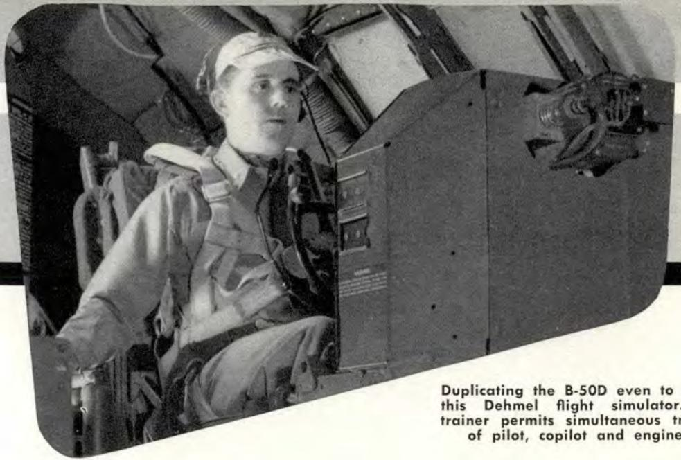
Duplicating the B-50D even to size is this Dehmel flight simulator. This trainer permits simultaneous training of pilot, copilot and engineer.
