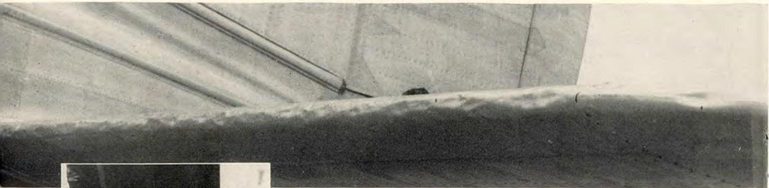
Above is a close-up of a hail-battered leading edge of a horizontal stabilizer showing what can happen to a plane flown through a thunderstorm area.
