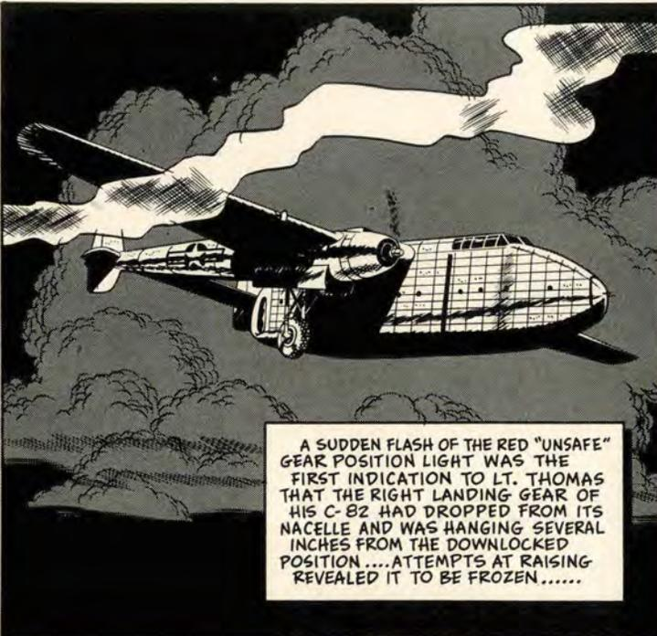
A SUDDEN FLASH OF THE RED "UNSAFE" GEAR POSITION LIGHT WAS THE FIRST INDICATION TO LT. THOMAS THAT THE RIGHT LANDING GEAR OF HIS C-82 HAD DROPPED FROM ITS NACELLE AND WAS HANGING SEVERAL INCHES FROM THE DOWNLOCKED POSITION ....ATTEMPTS AT RAISING REVEALED IT TO BE FROZEN.....
