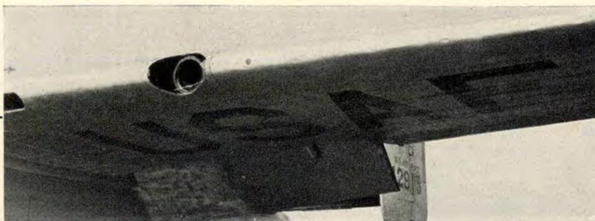
Heavy hail damage was incurred to this B-25 on both the leading edges of the wings between the two engine nacelles and the fuselage.
