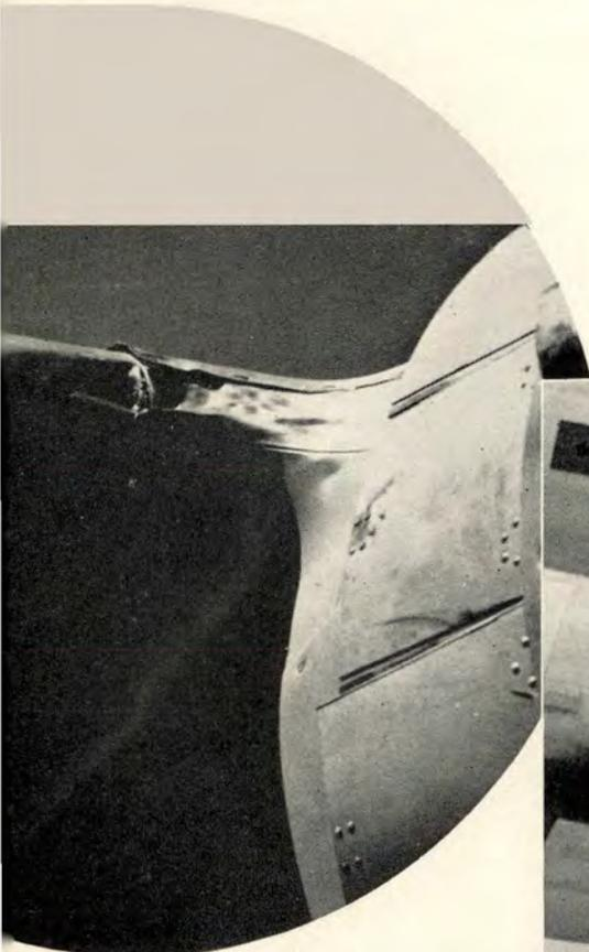
Cold front hail severely pock-marked the leading edge of this C-47 wing.
