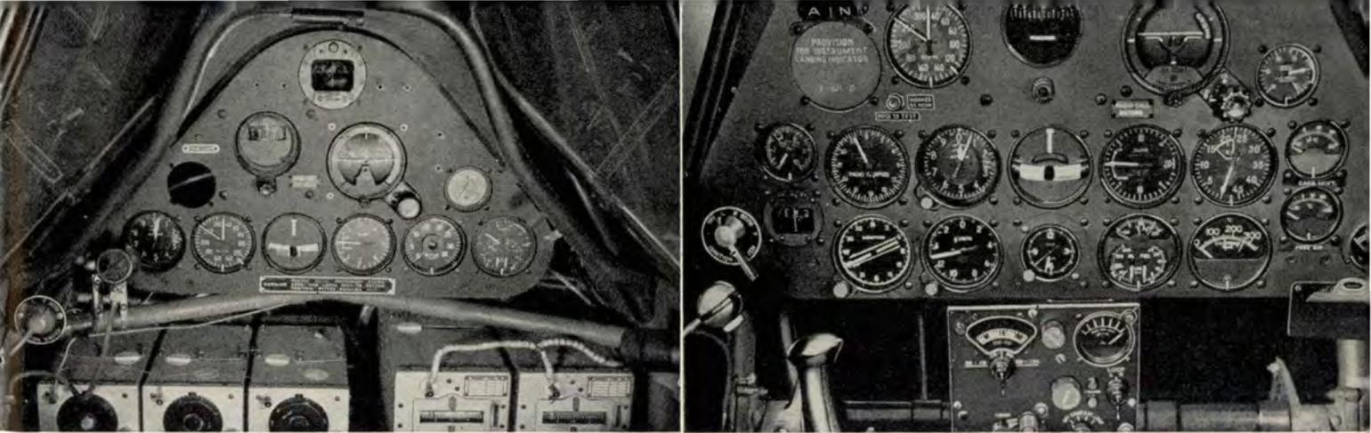
New equipment affects all aircraft. The rear cockpit of the T-6D, left, lacks the instrumentation of the T-6G, at right.
