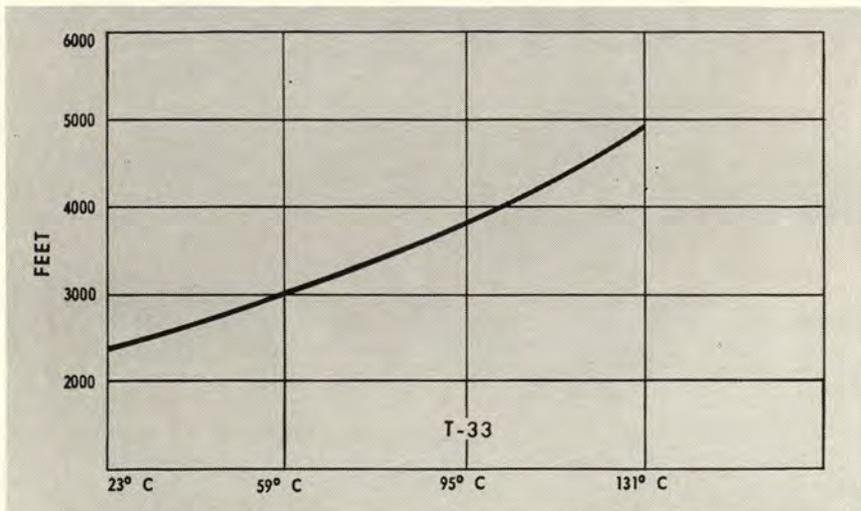
Increased temperatures mean it'll take more distance to get off the ground. In general, a twenty-degree rise in runway temperature means you will need about twenty per cent longer takeoff roll. The chart above shows the temperature-length ratio for a T-33. F-84C, below.
