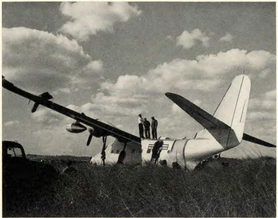
**This accident, brought about by an IP's late corrective action, resulted in the loss of an SA-16. Mission was a short field check-out.**
