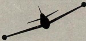
Approximately 20 degrees of bank necessary for a standard rate turn.
