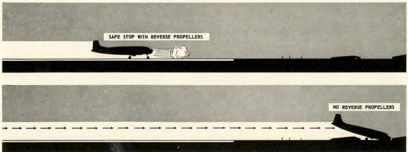
Power is best for keeping directional control—and for stopping if your airplane is equipped with reverse pitch propellers. The brakes, when used to slow the landing roll on slippery surfaces, should always be applied gently and cautiously. Right, a B-47 stops with aid of a drag chute. At light landing weights chute is not needed in a careful approach to long runways.
