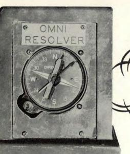
The instructor's standard C-8 Link direction indicator modified to become an Omni Resolver Simulator, This is used to help simulate Omni range approaches and cross countries.
