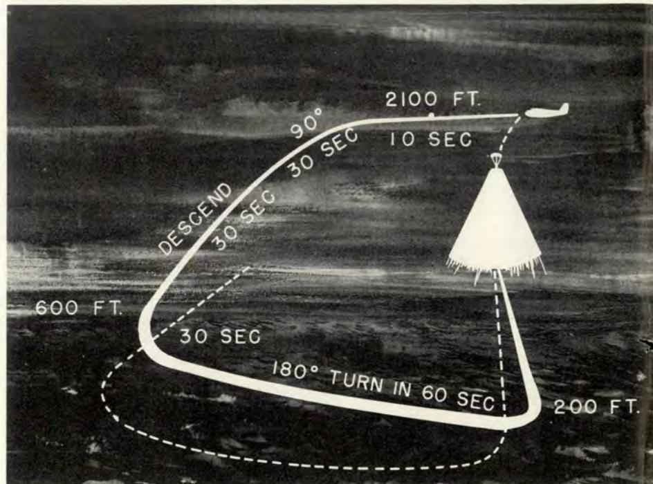
Recommended procedure when aircraft is ditched under its own flares.
