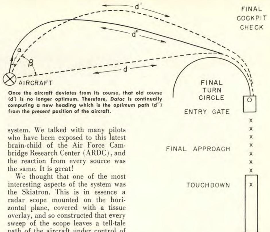
Once the aircraft deviates from its course, that old course (d') is no longer optimum. Therefore, Datac is continually computing a new heading which is the optimum path (d'') from the present position of the aircraft.
