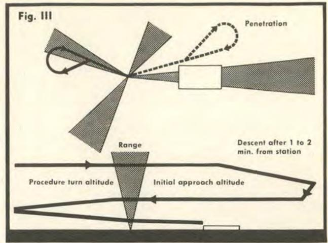
excess of 200 gallons. Descend to the altitude which will intercept the glide-path at the proper point. Then adjust the power to maintain altitude and airspeed. The amount of fuel used in this type of penetration and low approach for the T-33 will vary from 65 to 70 gallons.
