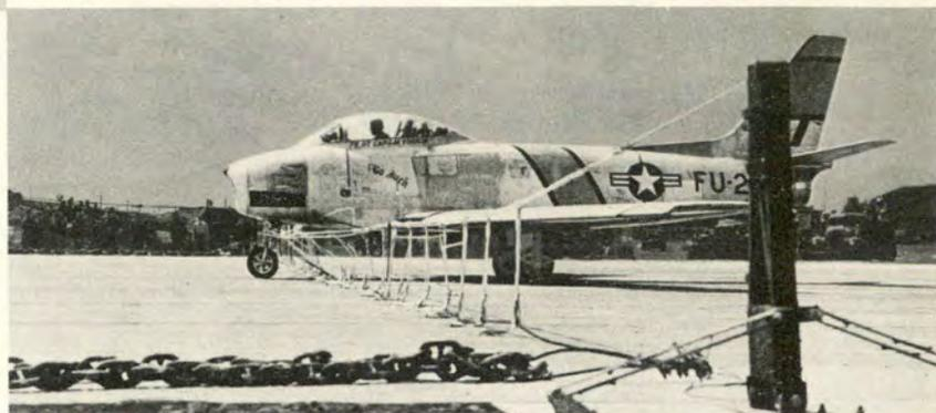
After nylon webbing is torn away by the nose gear and arresting cable has engaged the main landing gear, the pilot can expect the speed of the aircraft to diminish.
