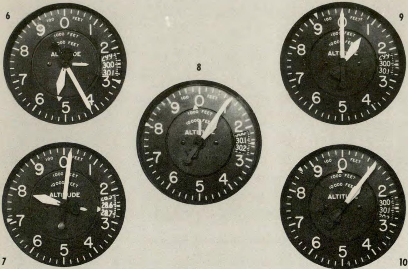
The problem seems to be that while a pilot is concentrating on flight attitude instruments, radio conversation and instrument procedures, that quick look at the altimeter often results in misinterpretation.
