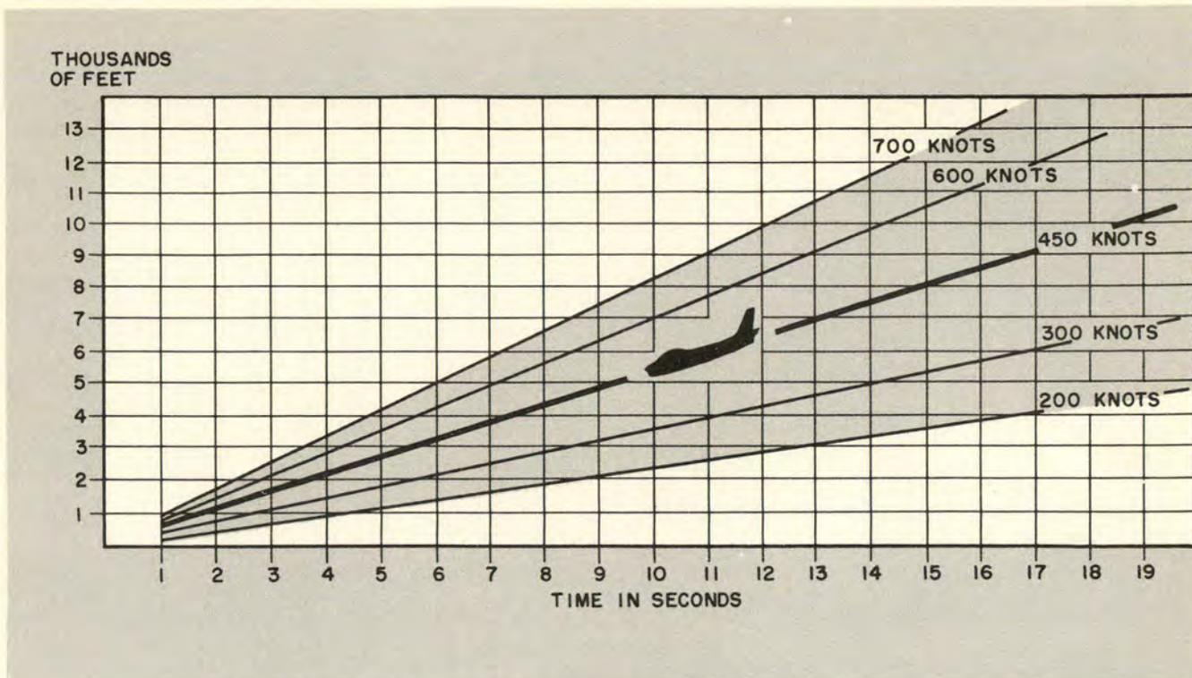
Chart A. As shown by the chart, at 450 knots in a 45-degree dive, 9000 feet will be lost in about 17 seconds.
