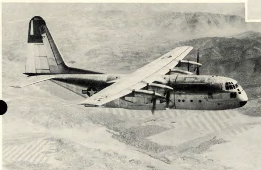
The new Lockheed YC-130, a turbo-prop aircraft designed as an all-purpose military transport.
