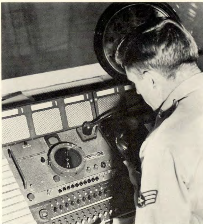
The DF operator gives a steer to the lost pilot and advises the evaluation net controller.
