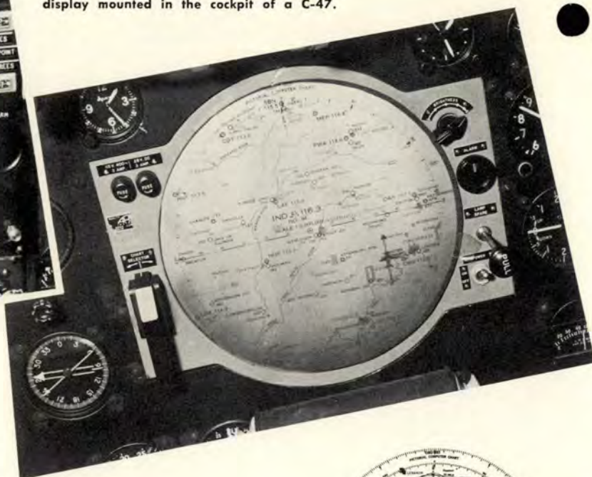
Left is the Type IVB pictorial display with a course line computer. Below is the Type V display mounted in the cockpit of a C-47.
