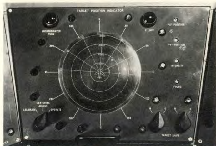
This indicator enables the instructor to position a target in relation to the student's simulator.
