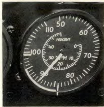
should re-group and give our rule-of-thumb yardstick some deep thought. The proposition, as outlined above, stating that thrust varies directly with RPM cubed can be most revealing. It can be applied to several phases of everyday jet operations.
