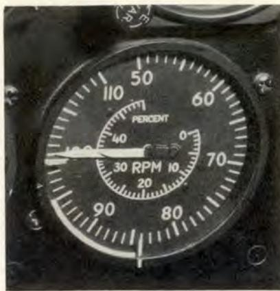
Using the rule of thumb, the power settings of 100, 90 and 80% of rpm, actually give only 100, 75 and 50% of available thrust.
