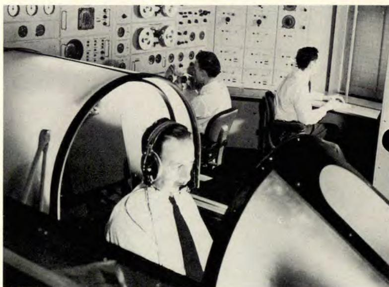
The F-89D Simulator in operation shows pilot, concentrating on his instrument panel, with radar instructor, upper left, and flight instructor checking and controlling the entire flight problem.
