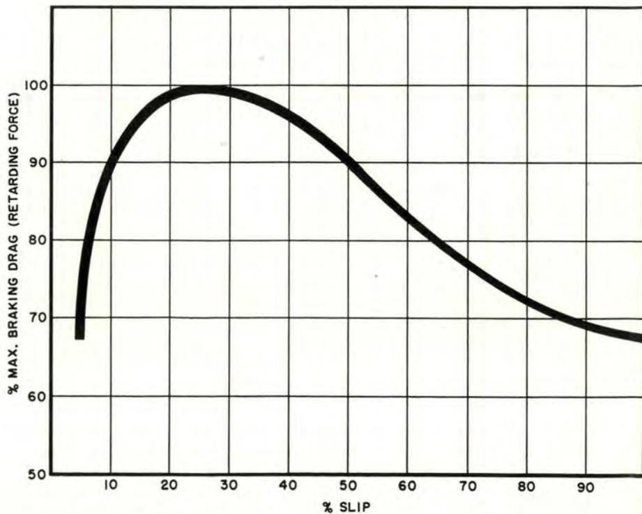
Figure 2. Note the effectiveness of braking versus tire slippage. Some slippage is needed.
