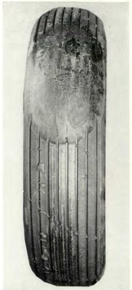
With the installation of anti-skid brakes, getting tires into this condition is almost eliminated.
