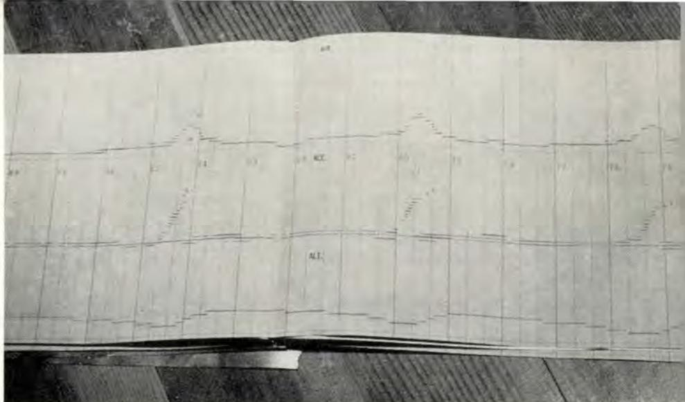
(G-forces). Others of a more elaborate type can record things like lift coefficient, Mach number, gust velocity, dive angles and so on. All of this is plotted on a continuous tape which rolls around at a given rate of speed and thereby gives all readings in terms of time. It will tell you exactly when you pulled 7G. Or for how many seconds during that dive you were doing this much airspeed and how long it took you to lose or gain this much altitude.
