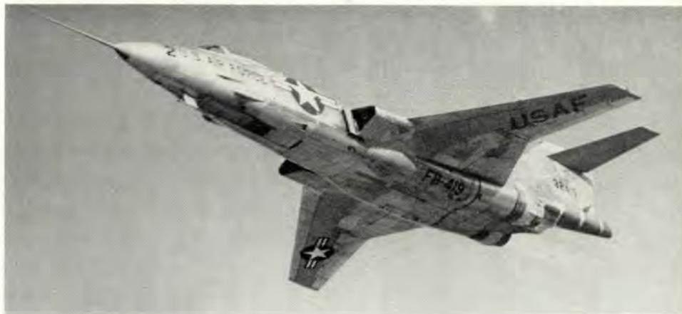
To maintain best climb speed, nose must be rotated steeply unless supersonic climb is desired.
