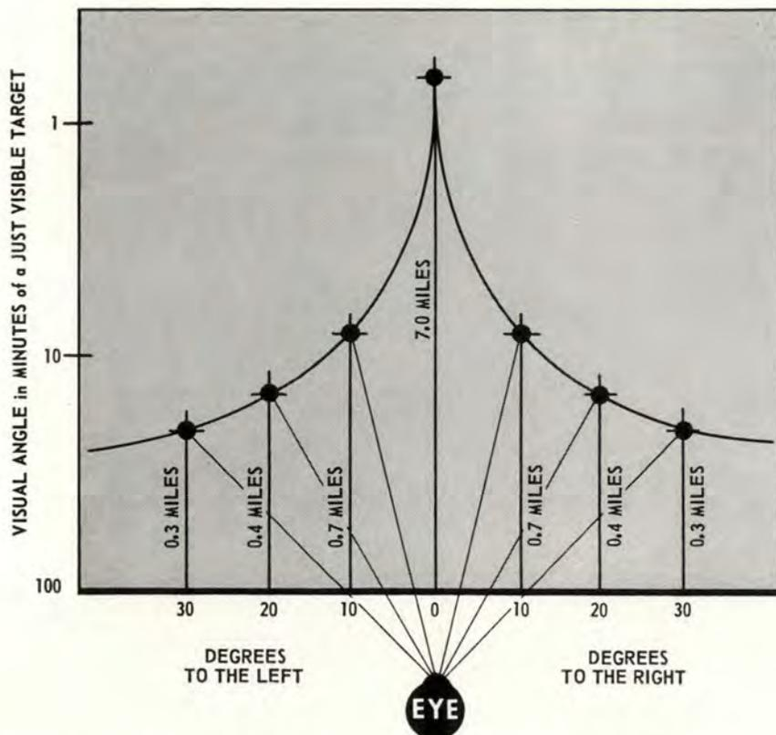
Figure 3. The effect of offset viewing angle on detection distance for fighter size aircraft.
