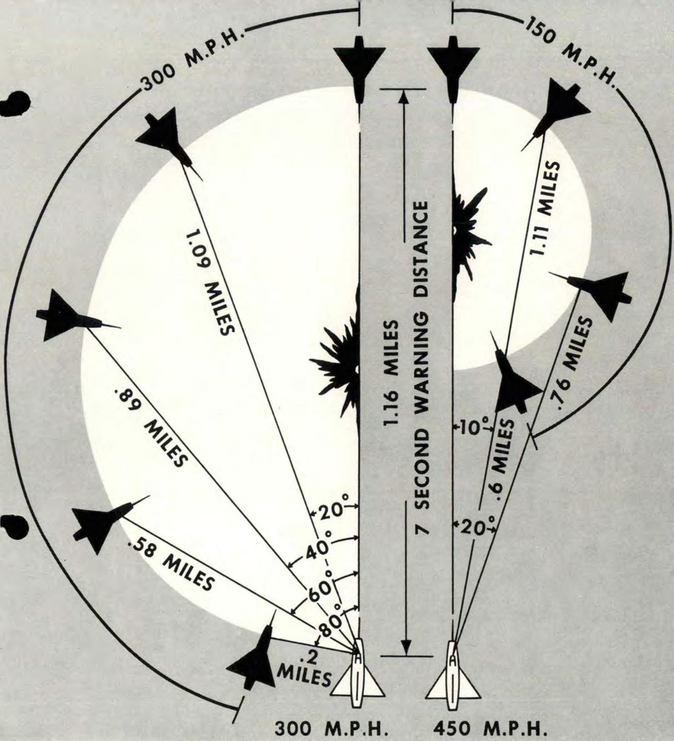
Figure 1. Distances at which other aircraft would appear seven seconds before collision for the two-speed combinations shown.
