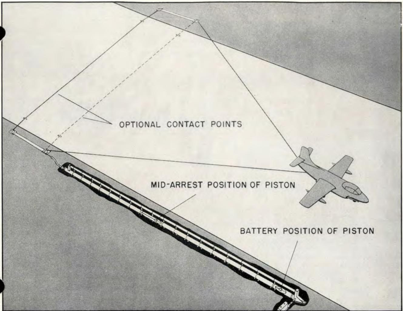
**A Squeeze Play**—A new method of landing jet fighters on short runways by “squeezing water” has been developed by the All American Engineering Company. It works this way: The landing aircraft engages the cables with a hook. The cable is attached to a piston in a water-filled pipe and upon engagement, the cable pulls the piston through the water, absorbing the energy created by the moving aircraft. Aircraft have been stopped within 100 yards without damage to the planes or the arresting gear.
