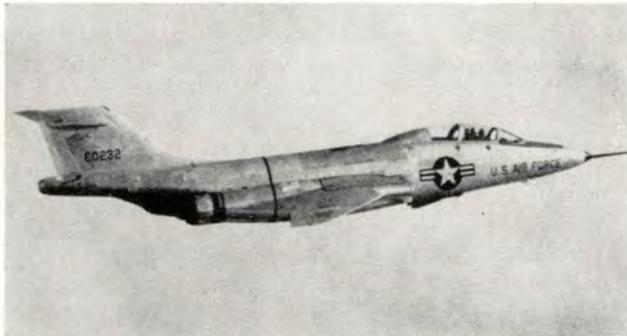
Above, is pictured the new, two-seat F-101B interceptor. It is one of three types of the Voodoo series designed for the Air Force.
