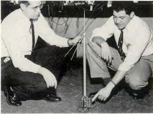
**Sardine Can**—A UHF Beacon Transmitter that fits into a standard size sardine can and a 12-inch tube that explodes into an antenna has been developed by Fairchild. Designed as an emergency signalling and communications device, the “sardine can” can be modified for voice or code. The transmitter weighs in at eight ounces and the hermetically-sealed tube is exploded into action by a gun powder charge.
