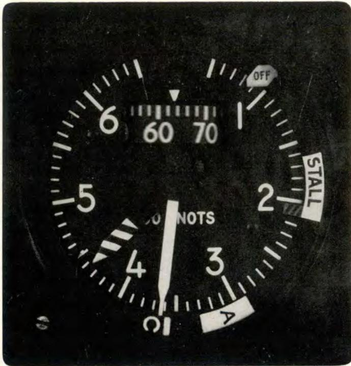
Here is the actual instrument. The various indices move around the outside of the dial. The indices are adjusted to the aircraft upon installation.
