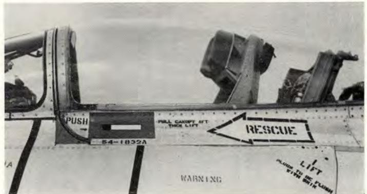
Shown here are two shots of the external release markings on the F-100A.
