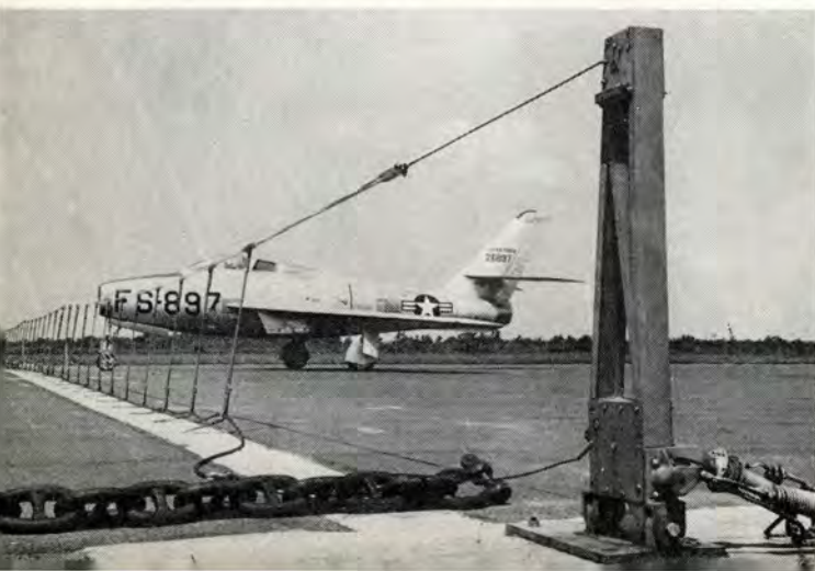
This F-84 is "clean" and set to make a successful barrier engagement.
