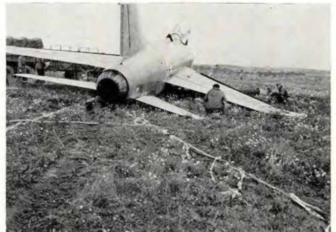
The best barrier in the world needs to have a stabilized overrun for good results. The one shown here was obviously too short for the job.
