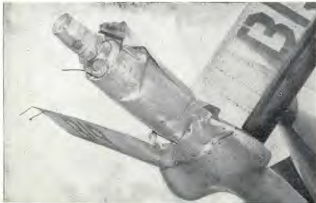
Left. This boom, jammed by a B-52, had its right ruddervator forced broadside to the airstream, rupturing the hydraulic system. The boom could then be neither hoisted nor flown up to the stowed position. Right, Sgt Jones in tail cone with the boom latching hook cable assembly.
