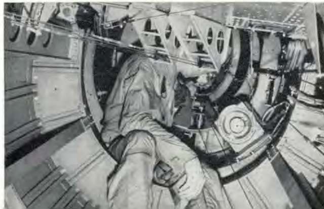
Left. This boom, jammed by a B-52, had its right ruddervator forced broadside to the airstream, rupturing the hydraulic system. The boom could then be neither hoisted nor flown up to the stowed position. Right, Sgt Jones in tail cone with the boom latching hook cable assembly.
