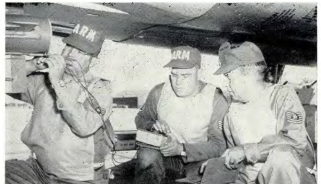
Above, SSgt F. L. Johnson, Sgt Karnicke, and SSgt Paul Drake load the Falcon on the missile launcher rail. Below, they make a stray voltage check to see that no voltage is leaking through the system.
