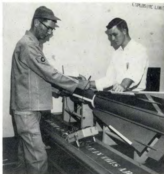
Below, SSgt G. W. Thomas, a missile guidance technician, runs a continuity check on the igniter circuit with the help of Mr. John E. Bunk, a Hughes tech rep. Note again the ever-present checklist.
