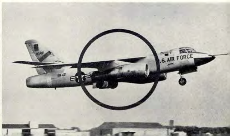
Pratt and Whitney TF33-P-7 engine during cold weather tests at Eglin, in flight on B-66 test bed.
