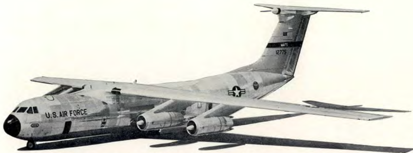
Four big engines providing 84,000 lbs. of thrust will push Air Force's new C-141A Starlifter.
