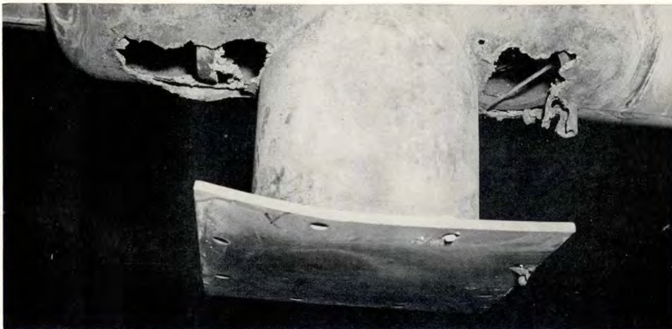
Large holes in LOX filter housing resulted from an internal oxygen-steel fire during missile downloading cycle.
