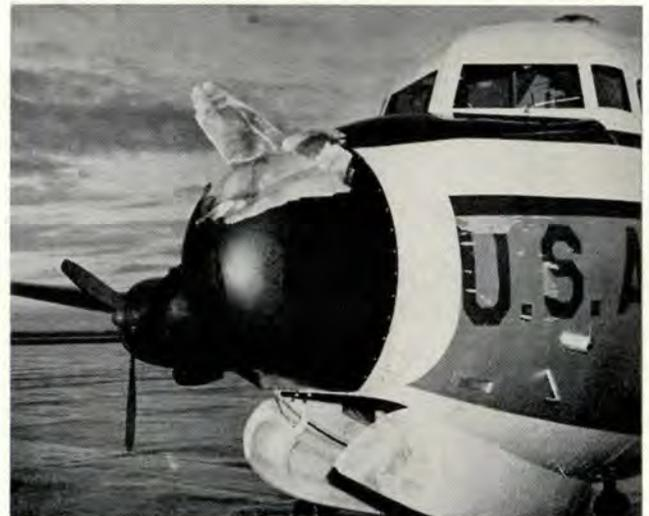
Lightning damage to radome of C-54
