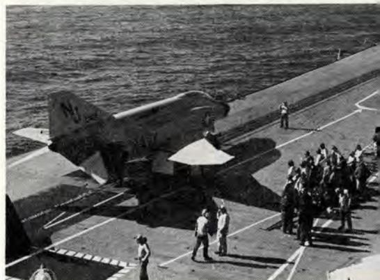
Plane aligned, bridle is attached.
