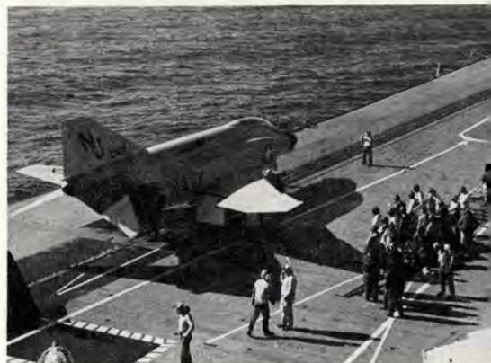
Plane aligned, bridle is attached.
