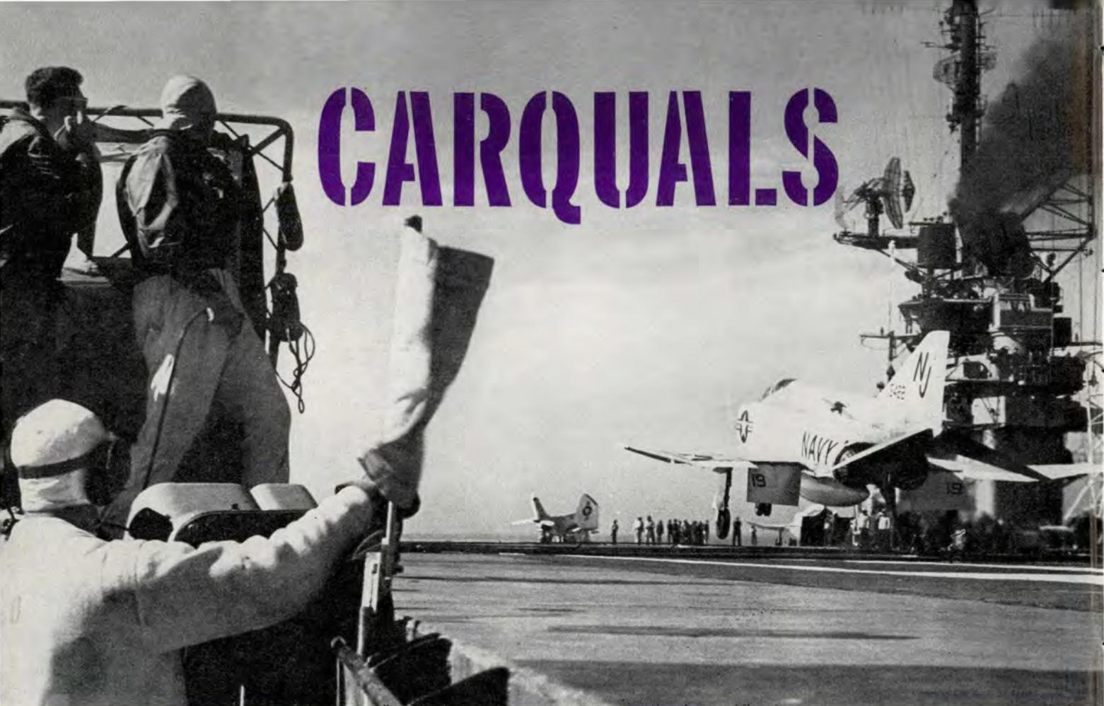
On a carrier qualification landing, a Navy pilot's F-4 is about to hook a wire.
