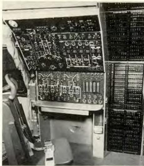
C-124, C-133 and C-135A engineers agreed that the panel on the C-141 is one of the best yet. Close location in relation to cockpit windows permits the engineer to aid in scanning. Photo is of mockup; aircraft panels differ slightly.
