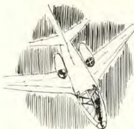
**SNOW BANKS AND ICE CHUNKS—** The co-pilot was taxiing the KC-97 from the left seat under supervision of the IP in the right seat. Moving down the ramp and heading for a taxiway, the right tip-tank struck a snow drift, damaging the tank and allowing fuel to spill out. The taxi line and snow drift had been clearly marked with red dye marker, but due to a sudden thaw the dye marker had become obliterated.
