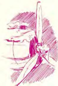
**GEAR UP BEFORE CLIMB ESTABLISHED-BELLY LANDING**—Recently a pilot retracted the gear before a climb was established and the aircraft settled back to the runway for a belly landing.
