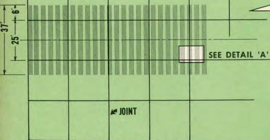
**NOTE: THE ENTIRE LENGTH OF THE RUNWAY WILL BE GROOVED WITH THE EXCEPTION OF SIX 25 ft. SECTIONS UNDER EACH BAK-12 PENDANT AND TWO ADJACENT 25 ft. SECTIONS.**
