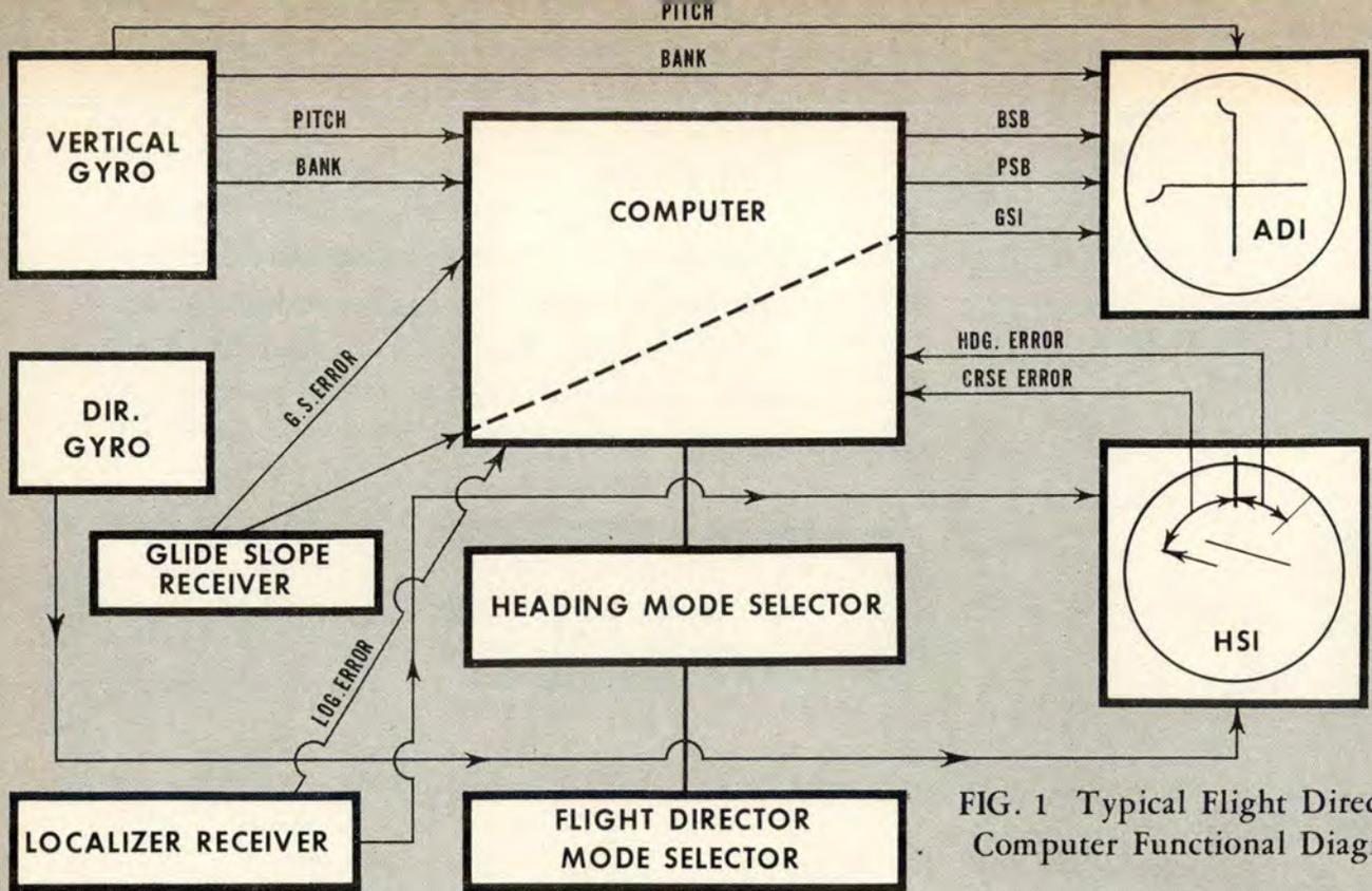
FIG. 1 Typical Flight Director Computer Functional Diagram
