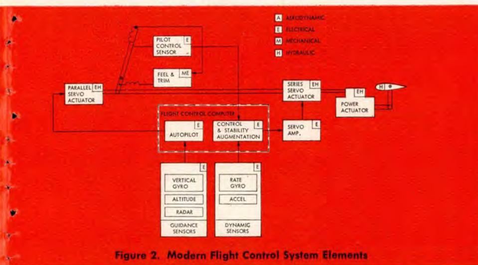
Figure 2. Modern Flight Control System Elements
