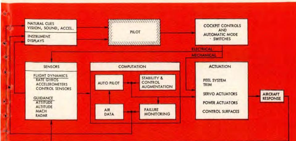
Figure 1. Relationship of Automatic and Pilot Flight Control Operations
