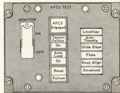
Automatic Flight Control System panel (left) located on center console. AFCS test panel (above) used to check terrain following and auto-landing modes.
