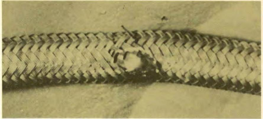
Results of improper clamping. Refer to TO 42E1-1-1 for limits of hose damage.
