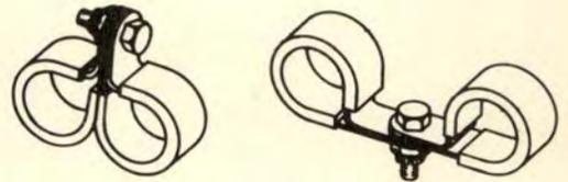
Installation of an Adel clamp to secure a wire bundle or a flexible line carrying fluid has always been difficult. Ask any old timer.
