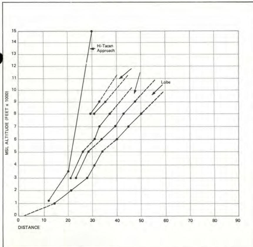
the antenna that produces the reflection. But that can't be done in the vicinity of the runway. Another complicating factor is the atmosphere and nearby obstructions. The atmosphere guides the radar wave in a path depending on the conditions at the time. This causes the lobes and nulls to change position. If conditions are severe enough, atmospheric holes can develop. Of course, nearby obstacles like trees or hangars on the horizon can hide an aircraft until it is above the line of sight.
