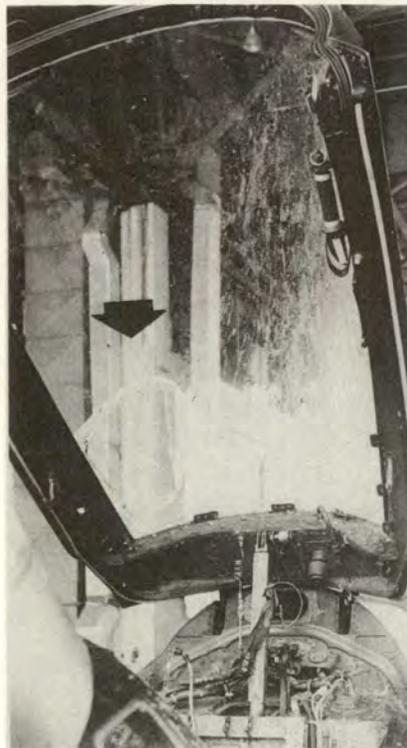
Left, rear canopy hole cut by firemen. Below, destructive force of impact damaged many components.
