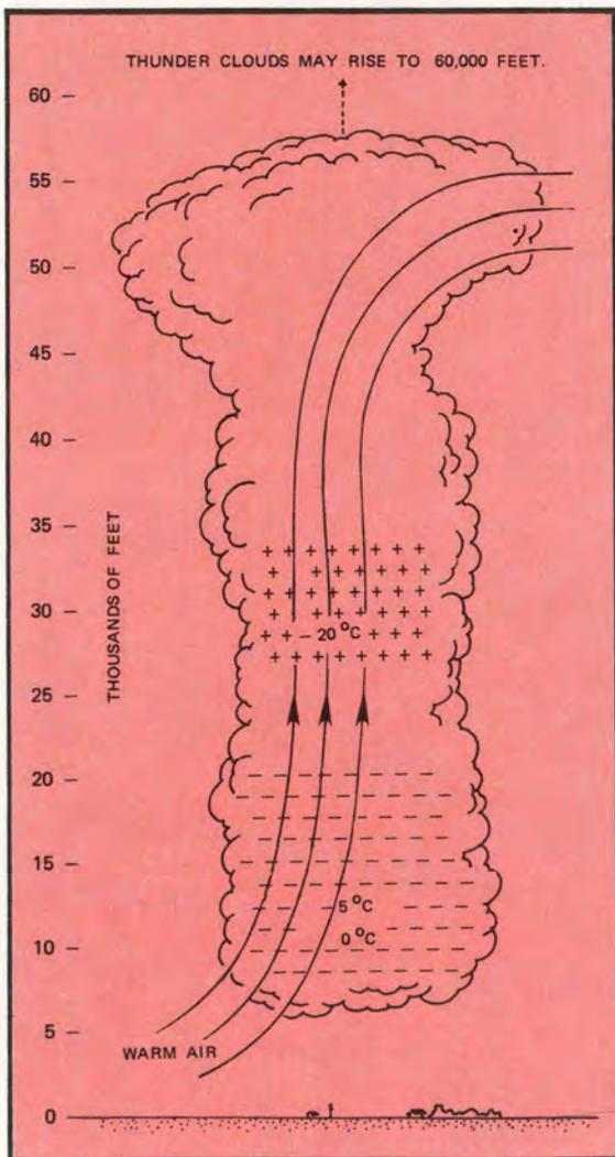
■ A lightning flash is a very long electrical spark which extends between one center of electrical charge in a cloud and another center of opposite polarity charge in the ground, in another cloud, or sometimes even in the same cloud. The energy that produces lightning is provided by warm air rising upwards into a developing cloud as shown in Figure 1.
