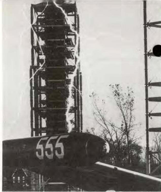
FIG. 13 Simulated lightning tests on wing-tip fuel tank at the GE High Voltage Laboratory, Pittsfield, Massachusetts.
