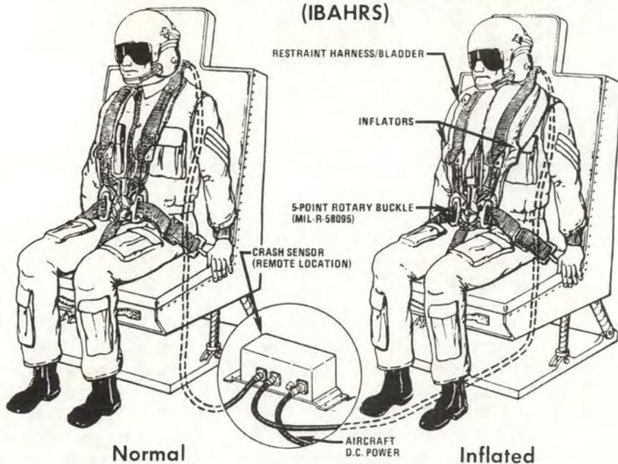
two of the factors described earlier—restraint and energy absorption. The restraint feature was a new inflatable body and head restraint system.
