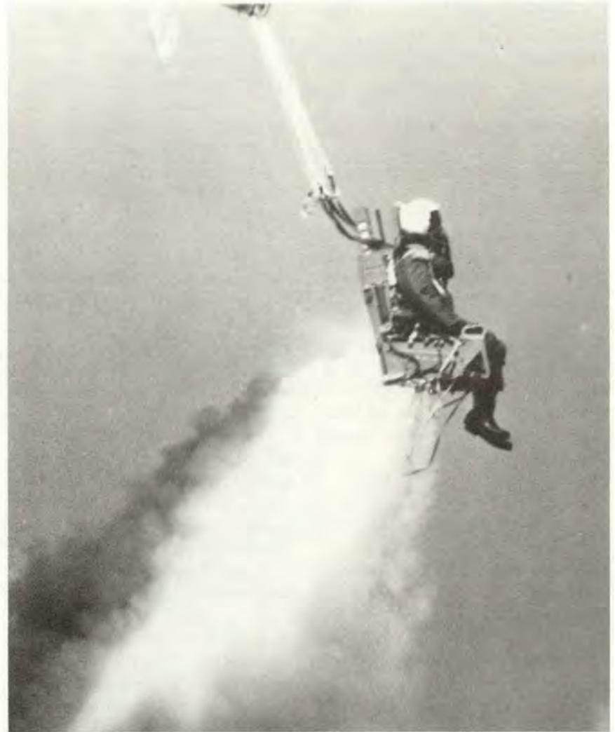
the release and are in the envelope, you can still reach back for your face curtain or lower ejection handle and eject.
