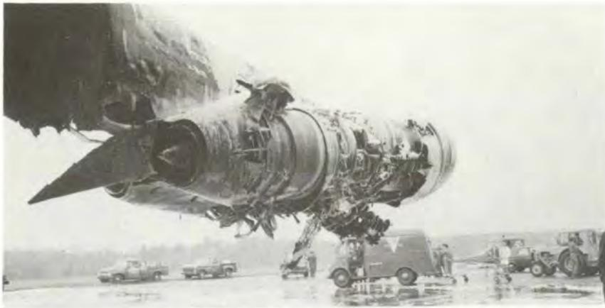
aircrew experienced torching on the engine and two overtemps which the pilot did not have investigated by maintenance. The engine turbine had been severely damaged by the overtemps. During flight, one of the blades failed. This caused extensive damage to the two adjacent engines as well as extreme vibration. The vibration caused the engine mounts on one engine to fail and resulted in actual loss of the engine from the aircraft.
