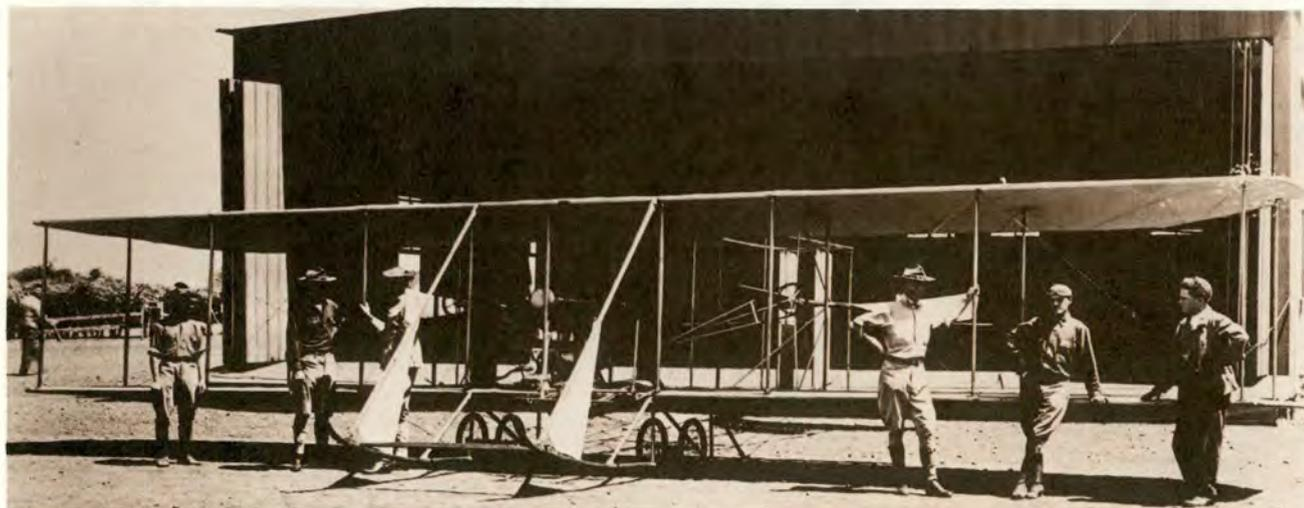
The Wright Model B included changes such as wheels, a rear-mounted elevator, and improved flight controls.
