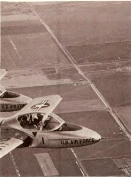
No Class B mishaps occurred in 1986. Nearly 210 Class C mishap reports received still show a high rate for engine failures/flameouts (48 Class Cs) and physiological incidents like hypoxia and GLOC (34 Class Cs). We are aware the engine tends to quit close to the edge of the performance envelope. Also, the nonavailability of a pressurized cabin and anti-G suit exposes T-37 crews to strenuous physiological demands.
