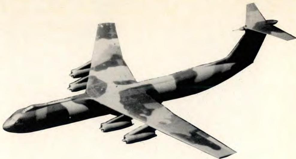
**Vertical T-Tail Loads** Recently, several aircraft have experienced vertical T-tail loads at or near design limit load (DLL) during low-level and air refueling operations. As a consequence, WR-ALC is working with Lockheed to develop a modification that will substantially strengthen the vertical spar of the T-tail. While all aircraft in the fleet will be modified, the first will be the SOLL II aircraft.
