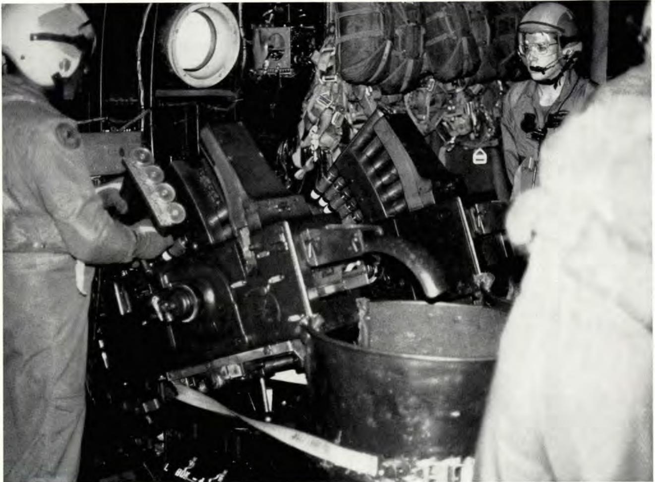
Pictured are aftgunners tending 40mm Bofors. The gunner feeds four-round clips of ammunition into the loader on top of the cannon while it is being fired.
