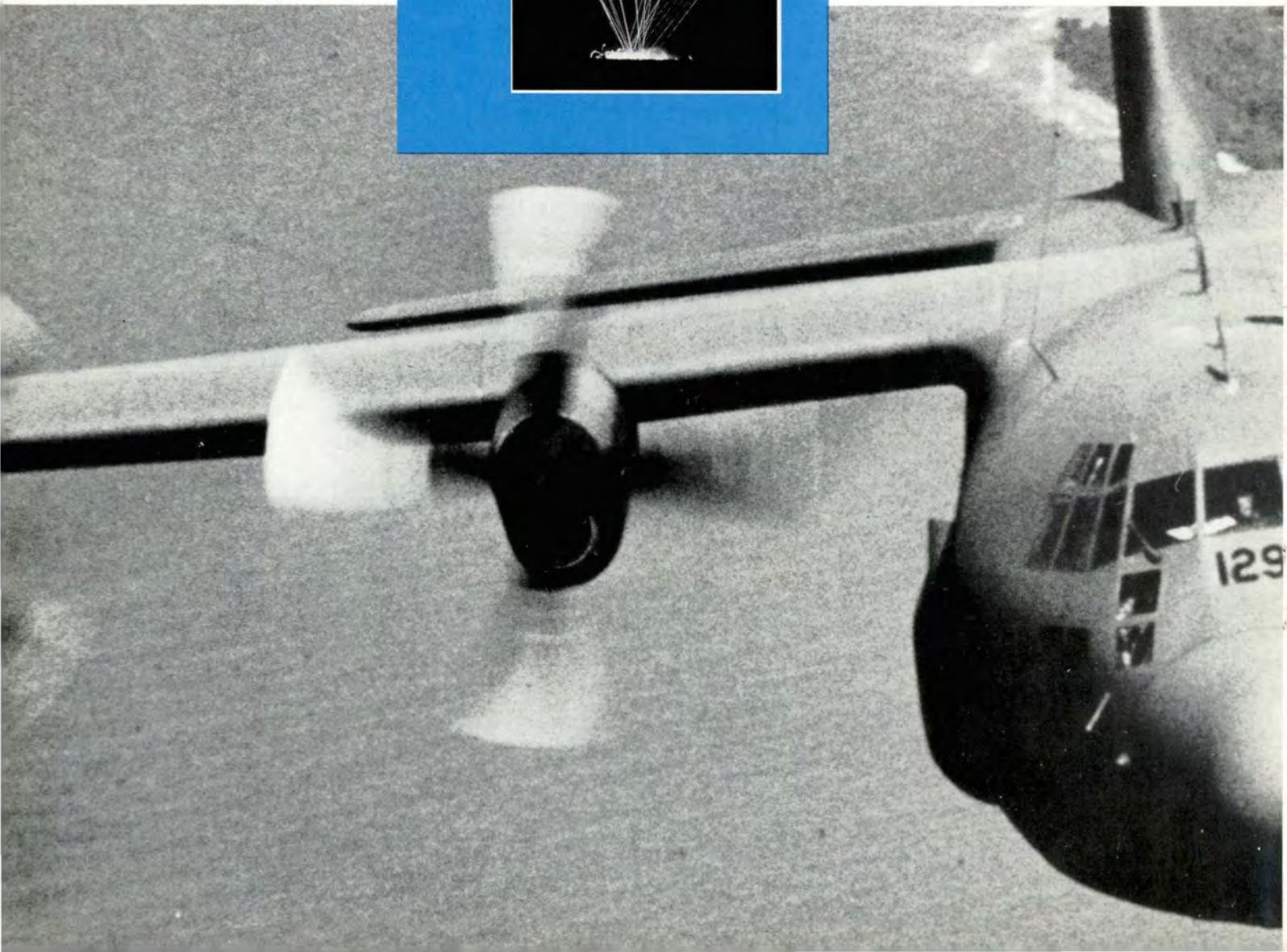
The AC-130A SPECTRE is a C-130 aircraft with a 17,000-pound modification. The mod added to the basic airframe is a weapons suite, a set of sensor systems, a fire control system, enhanced navigation and communications equipment, electronic combat equipment, and some light armor.
