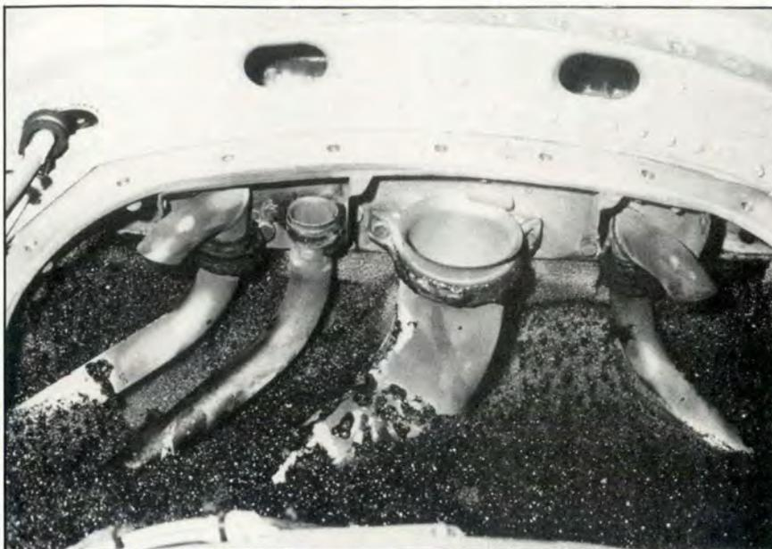
F-15 Fuel Tank No. 1 — Facts uncovered during the investigation indicate that the fire was not caused by a failure in one of the fuel tank's components. It was concluded that the inflight fire was the result of static electrical discharge in the vicinity of the four vent lines located in the forward portion of fuel tank. The fire was successfully contained by the suppression foam in the tank, damage was minor, and there was no apparent impairment of fuel system operation.
