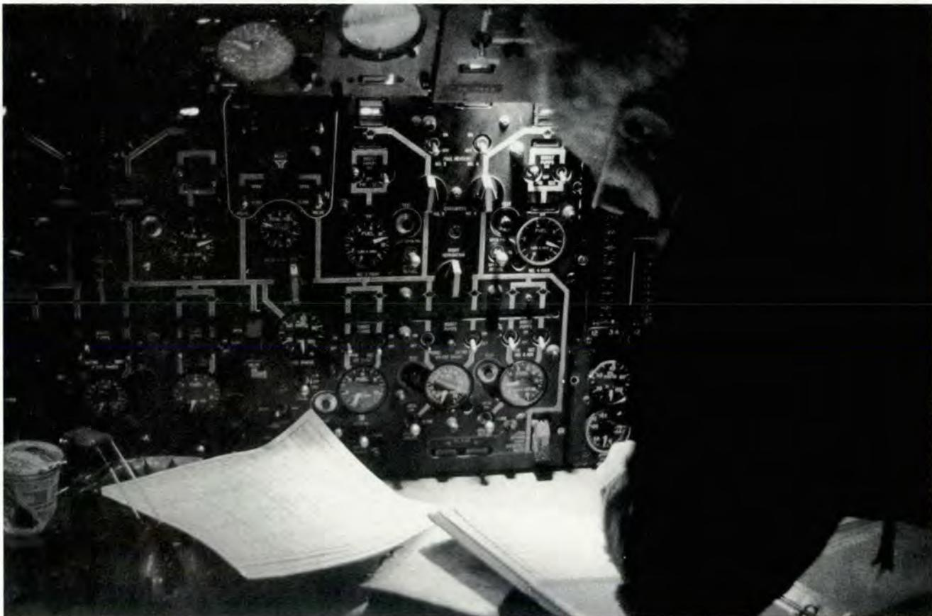
"When I do a full preflight," explained TSgt Richter, "I check all the flight controls to make sure they're doing what they are supposed to, ensuring there is no binding. I also make sure the hydraulic systems are working properly. I make sure all of the system warning lights are working, and functionally check the brakes for their proper application sequence."
