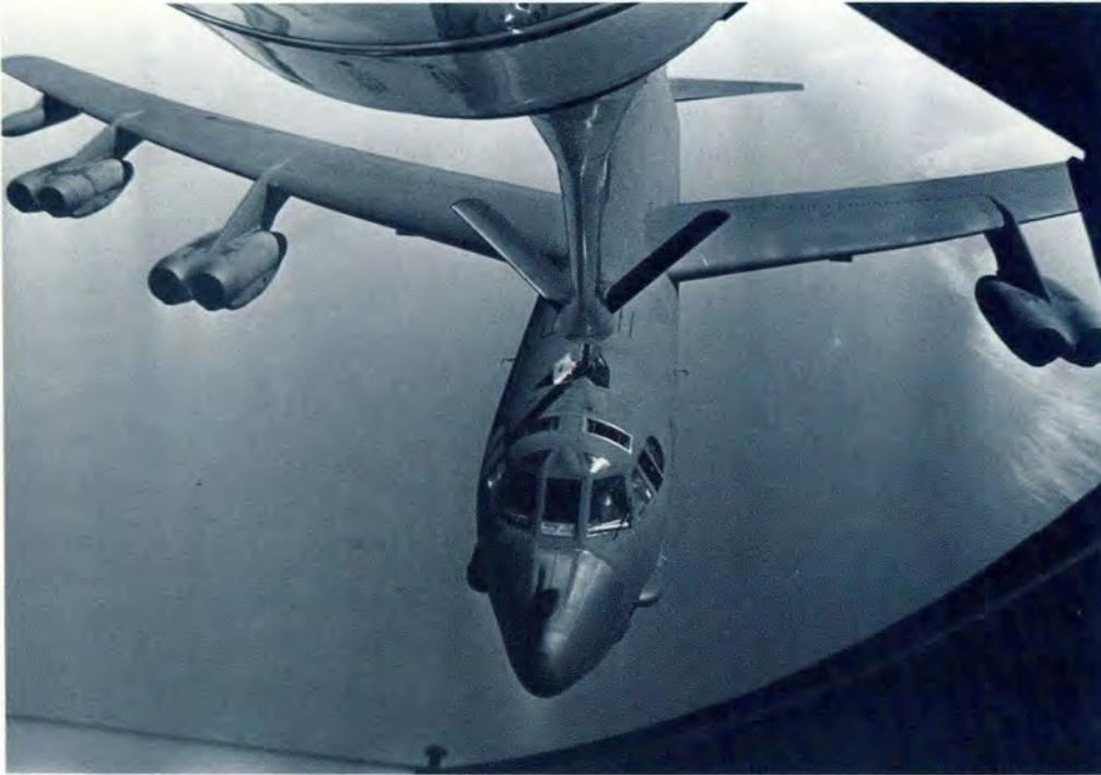
A B-52G receives fuel from the boom of a KC-135 tanker.
