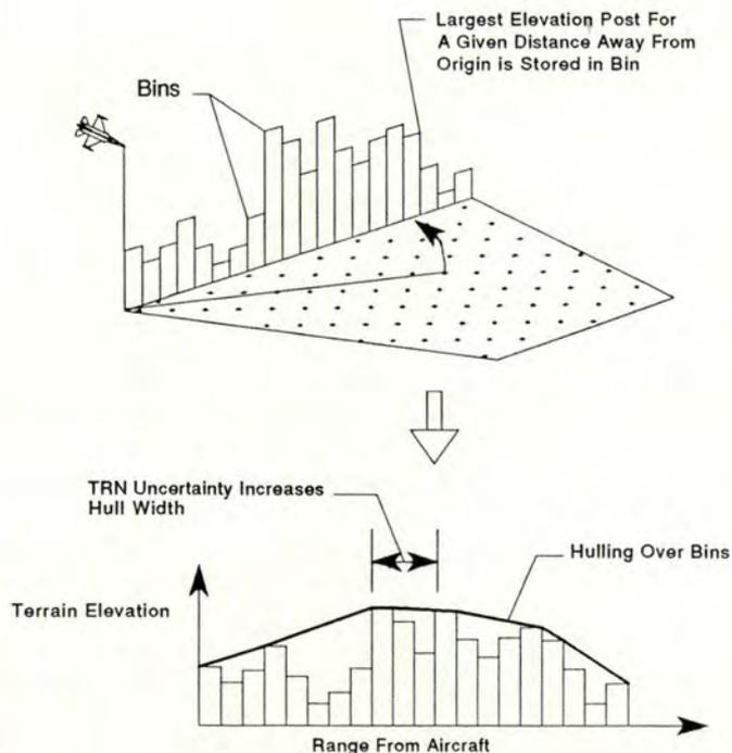
**Figure 2** ■ Binning and Hulling Process
