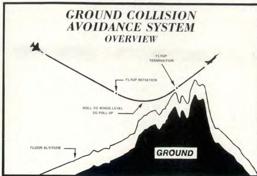
The GCAS computer constantly calculates altitude needed to recover above the floor altitude. The system begins warning the pilot visually and aurally 5 seconds before taking control. If the pilot doesn't respond, the GCAS performs a flyup maneuver at the last second.
