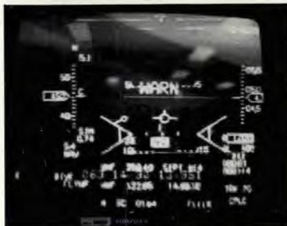
Everyone in the control room carefully monitors the test profile as the chevrons come together indicating time to flyup.
